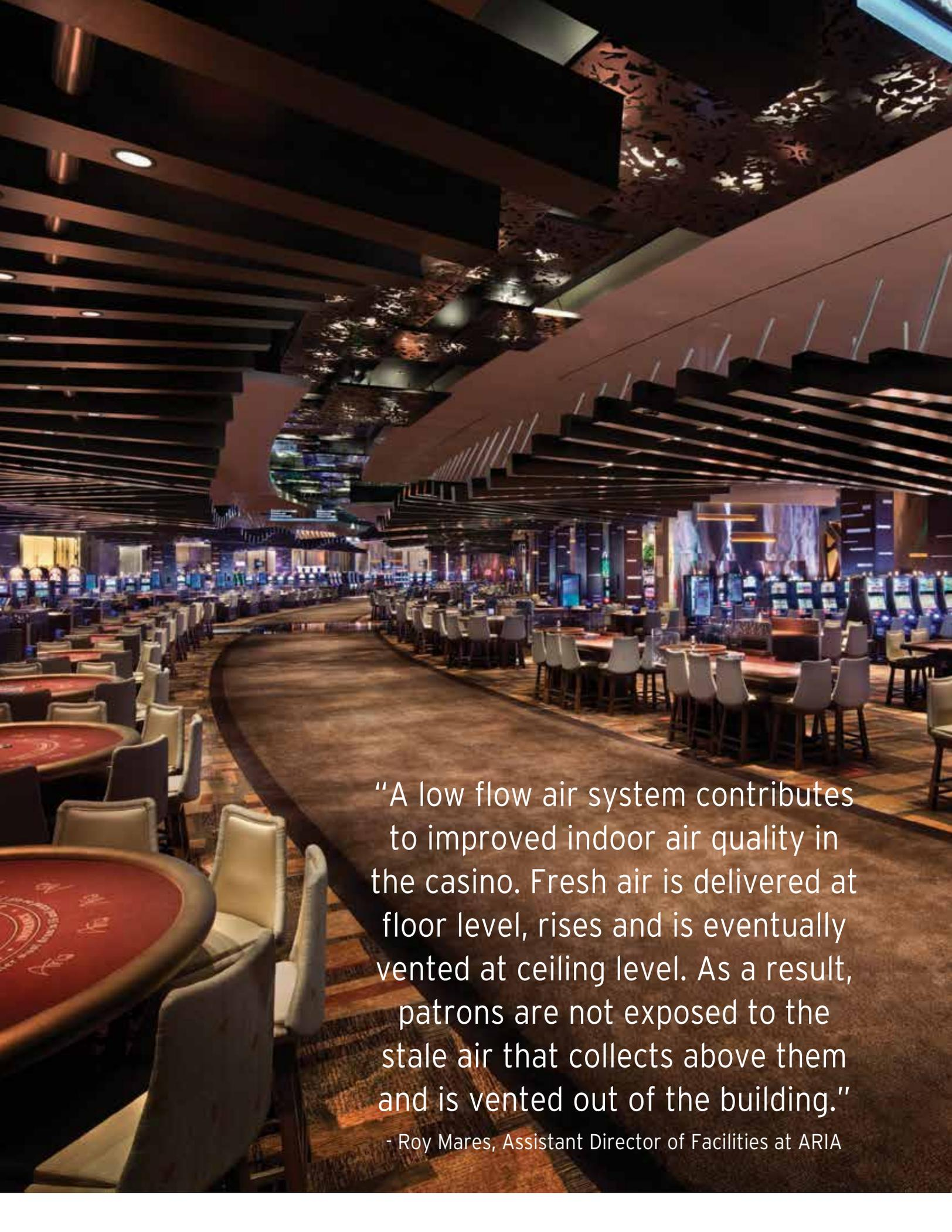
“A low flow air system contributes to improved indoor air quality in the casino. Fresh air is delivered at floor level, rises and is eventually vented at ceiling level. As a result, patrons are not exposed to the stale air that collects above them and is vented out of the building.”
